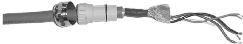
Figure 14 Applying the heat shrink
